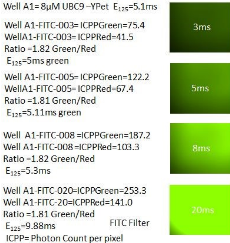
Figure 5.8: The methodology for finding the effective exposure at constant intensity of 125. For Well A1 the E 125 = 5.1 ms.
