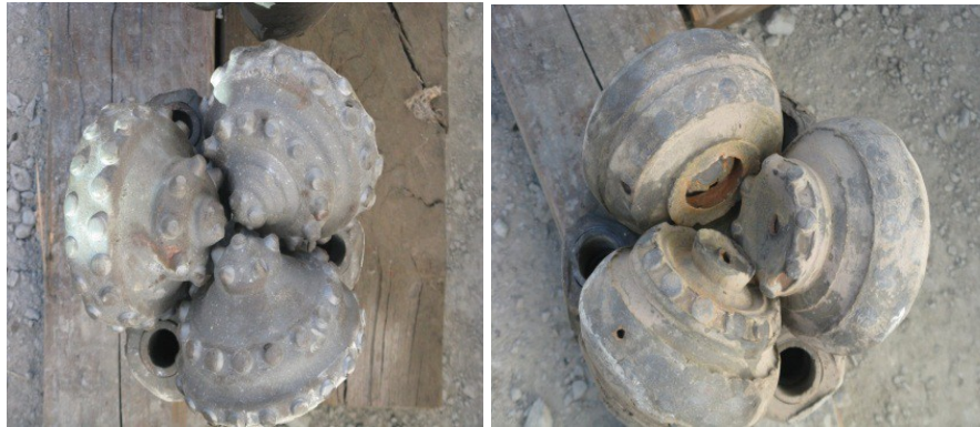
735 Figure 11: Average bit condition after 91.4 m (300 ft) of typical air drilling in the normal temperature 736 Geysers reservoir (left) and Prati 32 final bit condition after 30.5 m (100 ft) of air drilling to a final 737 depth of 3396 m (11143 ft) in the high temperature reservoir.
