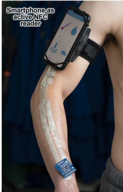
Fig. 70. The nearfield propagation can be seamlessly routed along and between the epidermal and textile-integrated from factors, enabling multi-purpose applications.
