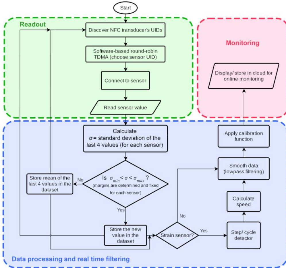
Fig. 34. Flowchart for software based TDMA and sensor data processing. The sensor value storage decision (based on the standard deviation) allows for holding the sensor values close to the previously logged data, ultimately rejecting artifacts caused by the analog sensor noise in real time and without inducing considerable latency. The SD margin and calibration function is unique to each sensor type and does not change throughout the monitoring process.
