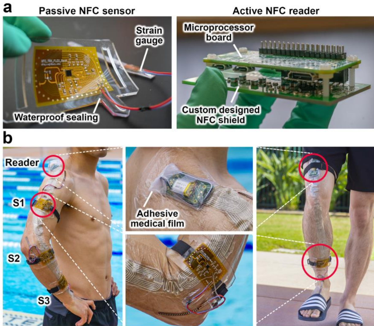
Fig. 68. Amphibius epidermal BAN functioning in a wide span of challenging environments. (a) The passive flexible sensor board with an integrated strain gauge and miniature active NFC reader. (b) Integration of epidermal skin patches on the human body to transmit wireless power from the NFC reader to the local sensors and collect motion data.
