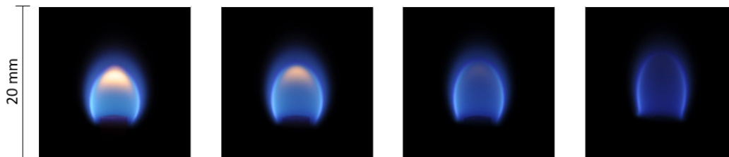
Figure 1.1: Laminar water-laden methane/air coflow flame at different water dilution levels: X_{\text{H}_2\text{O}} = 0, 0.2, 0.4, 0.6 .
