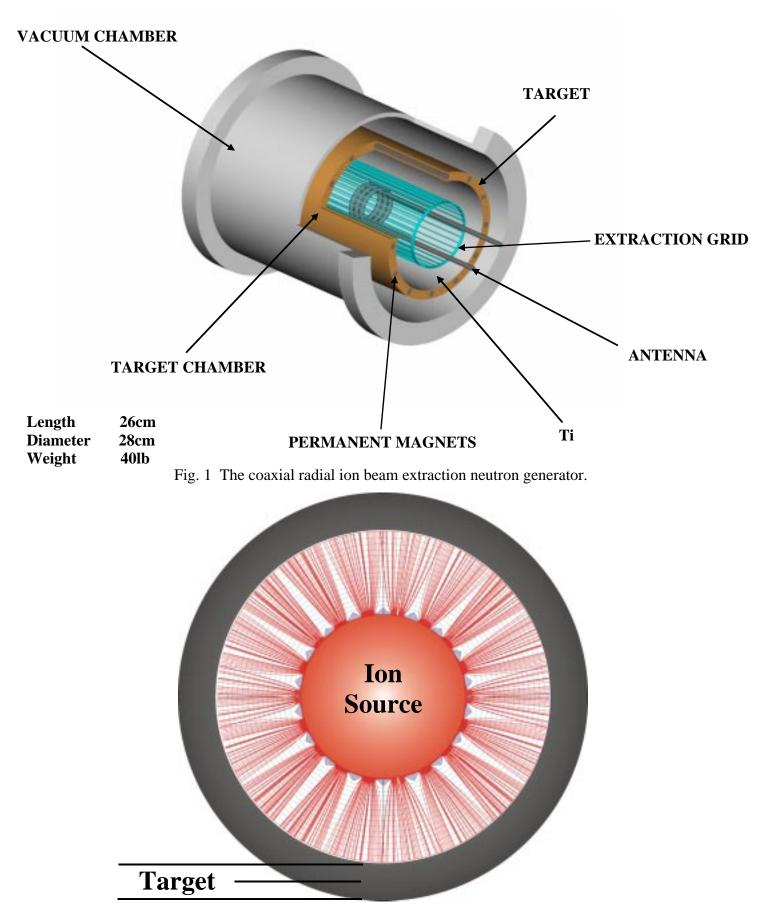
Fig. 2 Cross-sectional view of the coaxial neutron generator with ion beam trajectories computed by using the IGUN simulation code.
