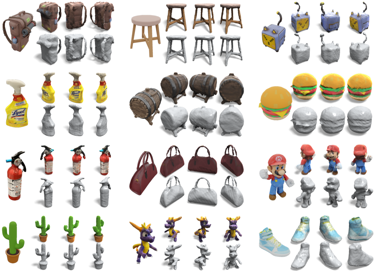
Figure 2.1. One-2-3-45 reconstructs a full 360° mesh of any object in 45 seconds given a single image of it. In each example, we showcase the input image in the left column, alongside the generated textured and textureless meshes from three different views.
