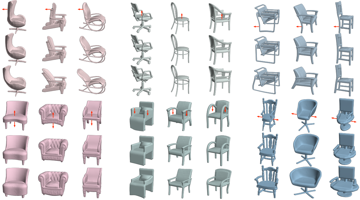
Figure 4.9. Learned meta-handles across different shapes. The figure includes six meta-handles, and each color indicates a distinct one. For each meta-handle, the figure demonstrates the corresponding deformations on three different shapes, with the red arrows highlighting the deformation direction. The meta-handles are consistent across various shapes.
