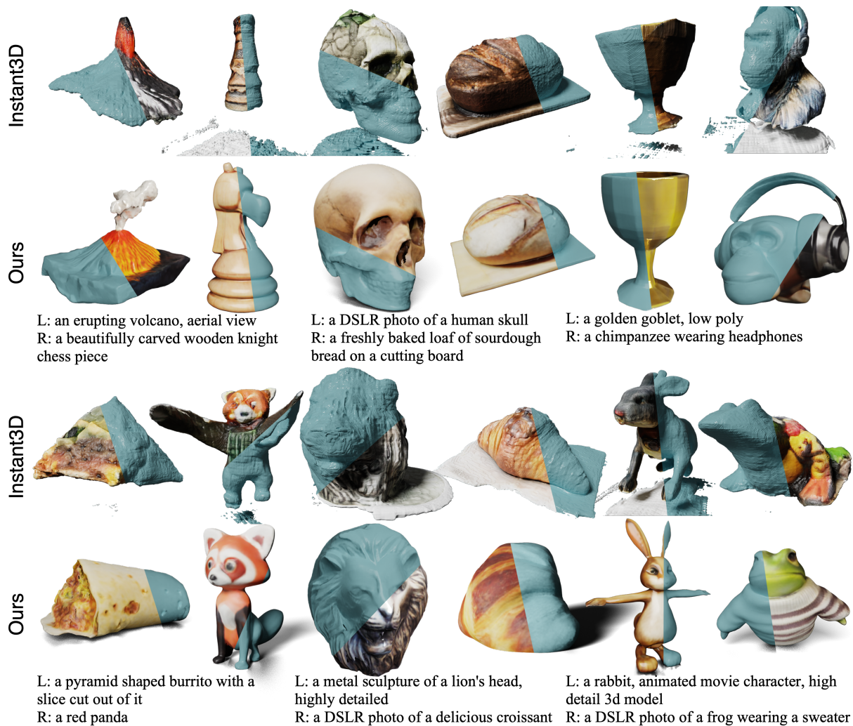
Figure 4.4. Application: Text to 3D. Given a text prompt, a 2D diffusion model first predicts multi-view RGB and normal images, which are then fed to MeshFormer for 3D reconstruction.
