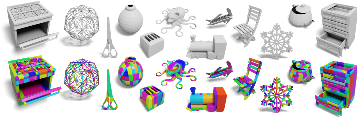
Figure 6.10. CoACD decompose a solid mesh into a set of components and utilize the convex hulls of the components (shown in different colors) to represent the original shape. Compared to prior works, we can better capture the fine-grained structures of the input shape with fewer components. See handles of the oven and the cabinet, slots of the toaster, and the spout of the kettle (zoom in for details). The high-quality decomposition enables delicate object interaction in downstream applications (e.g., a robot opens the drawer by grabbing the handles).
