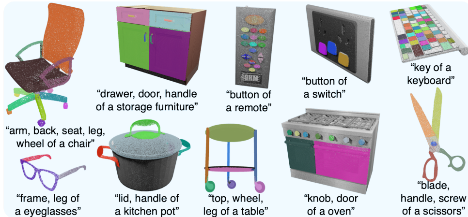
Figure 6.6. Instance segmentation results of our method (8-shot) on the PartNetE dataset. Different part instances are in different colors (zoom in for details).
