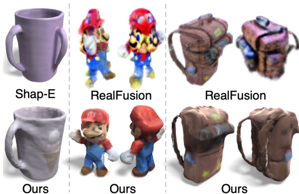
Figure 2.7. Unlike previous approaches, One-2-3-45 doesn't suffer from the multi-face problem (Janus problem).
