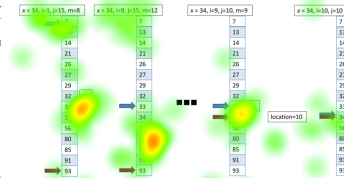
Figure: A run through binary search with x=34 . The result of the binary search on the sorted list is location=10 .
