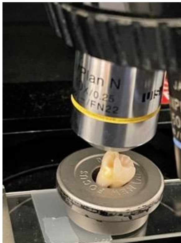
Figure 7. Tooth Mild Center (TMC) stabilized on metal piece to collect spectra.
