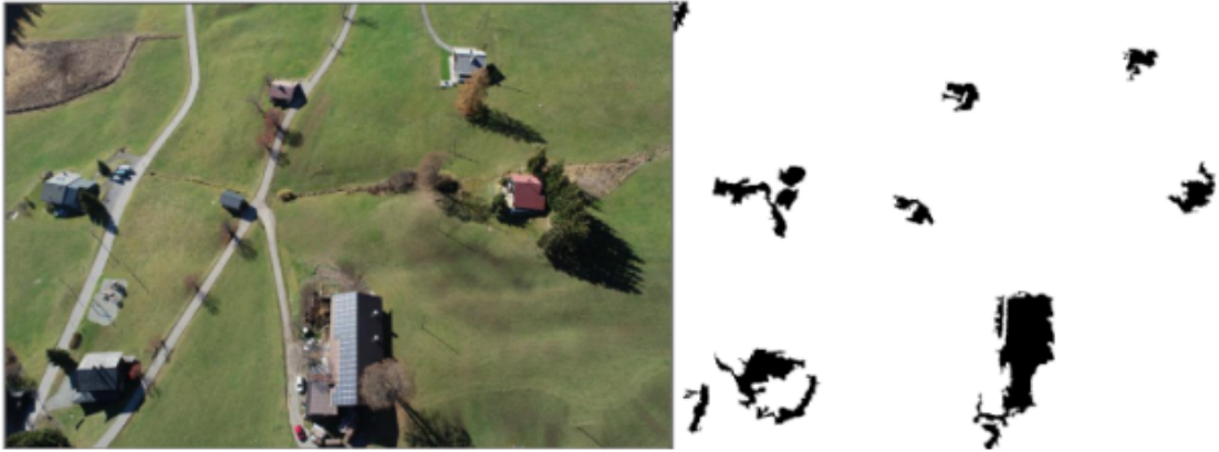
Figure S4. ACCT applied on image of aerial photography. An image taken from a public dataset by Yan et al. with permission granted under MIT license. The image consists of houses in a field along with the image segmented for houses by ACCT. a threshold of 0.5 was used with a minimum pixel size for objects of 300 and maximum of 1000. The segmentation shows the rough positions or irregularities in the landscape, demonstrating the potential of ACCT outside the biological context.
