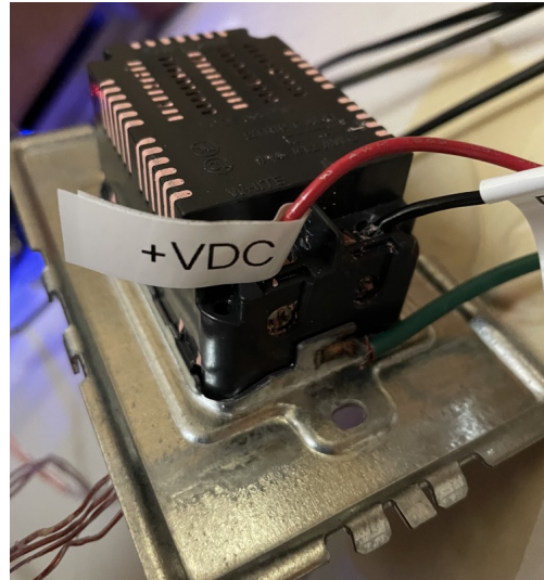
Fig. 3. The 140 W USB-C outlet prototype and Legrand Adorne faceplate.
