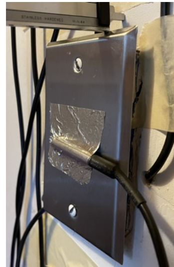
Fig. 6. The mock-up mounted in the wall section, with a 1 cm gap between the faceplate and wall.
