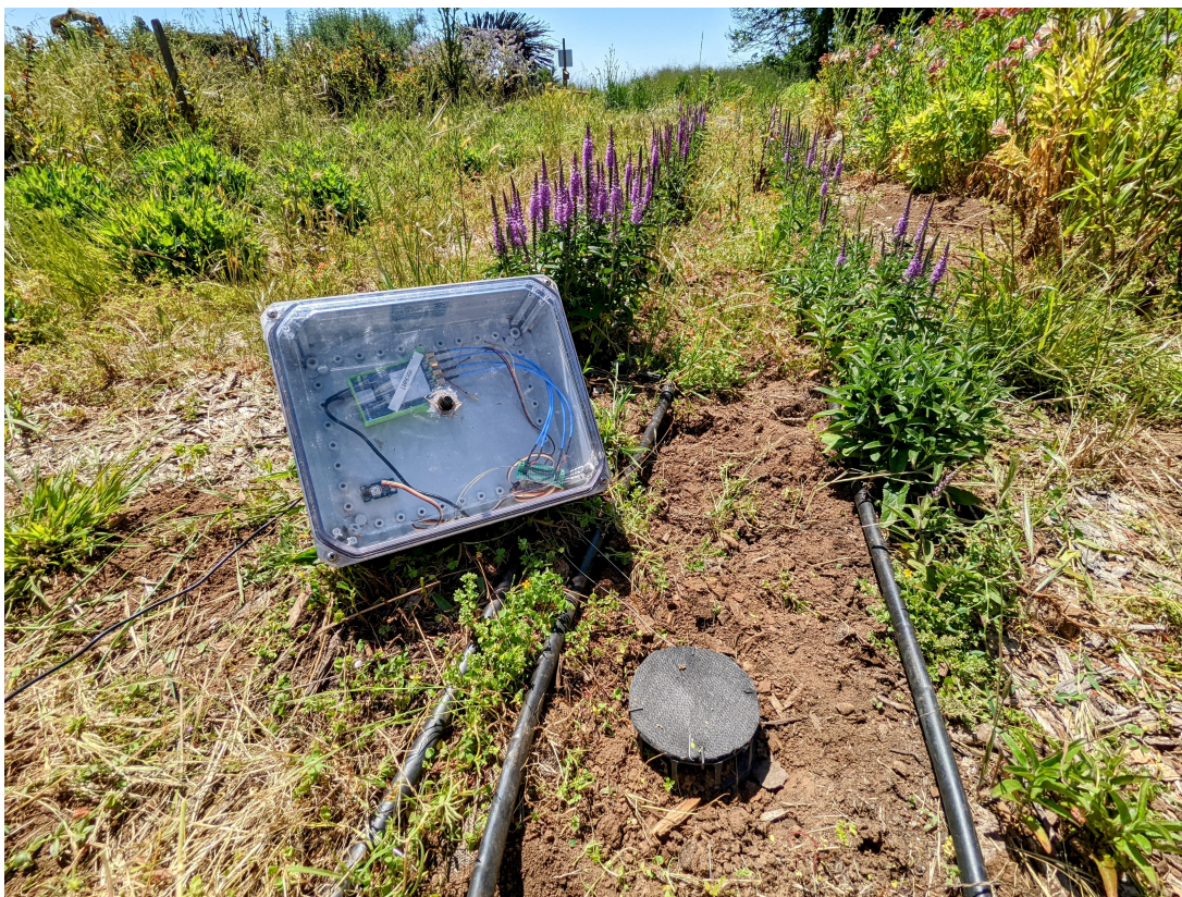
Figure 1: Soil microbial fuel cell staged for deployment at the University of California, Santa Cruz Center for Agroecology.
