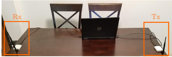
Figure 6.5: Over-the-air capture setup using USRPs B205 mini.
