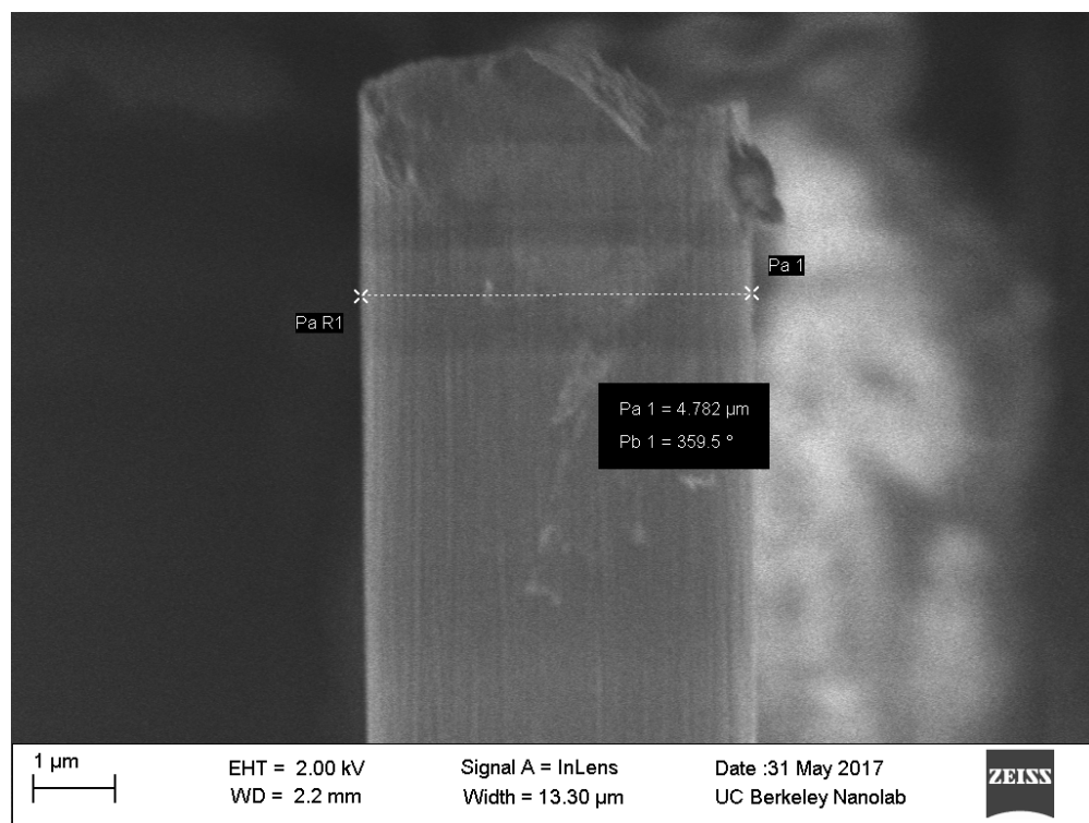
Figure 1.8: SEM of a 4.8 \mu\text{m} carbon fiber.
