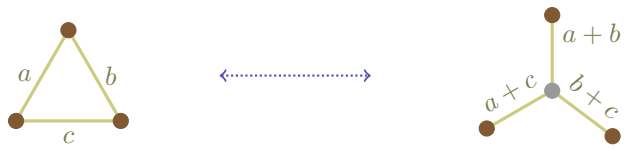
Figure B.2: The new entropy-preserving graph operation \Delta -Y. Vertices are color-coded as in fig. B.1.
