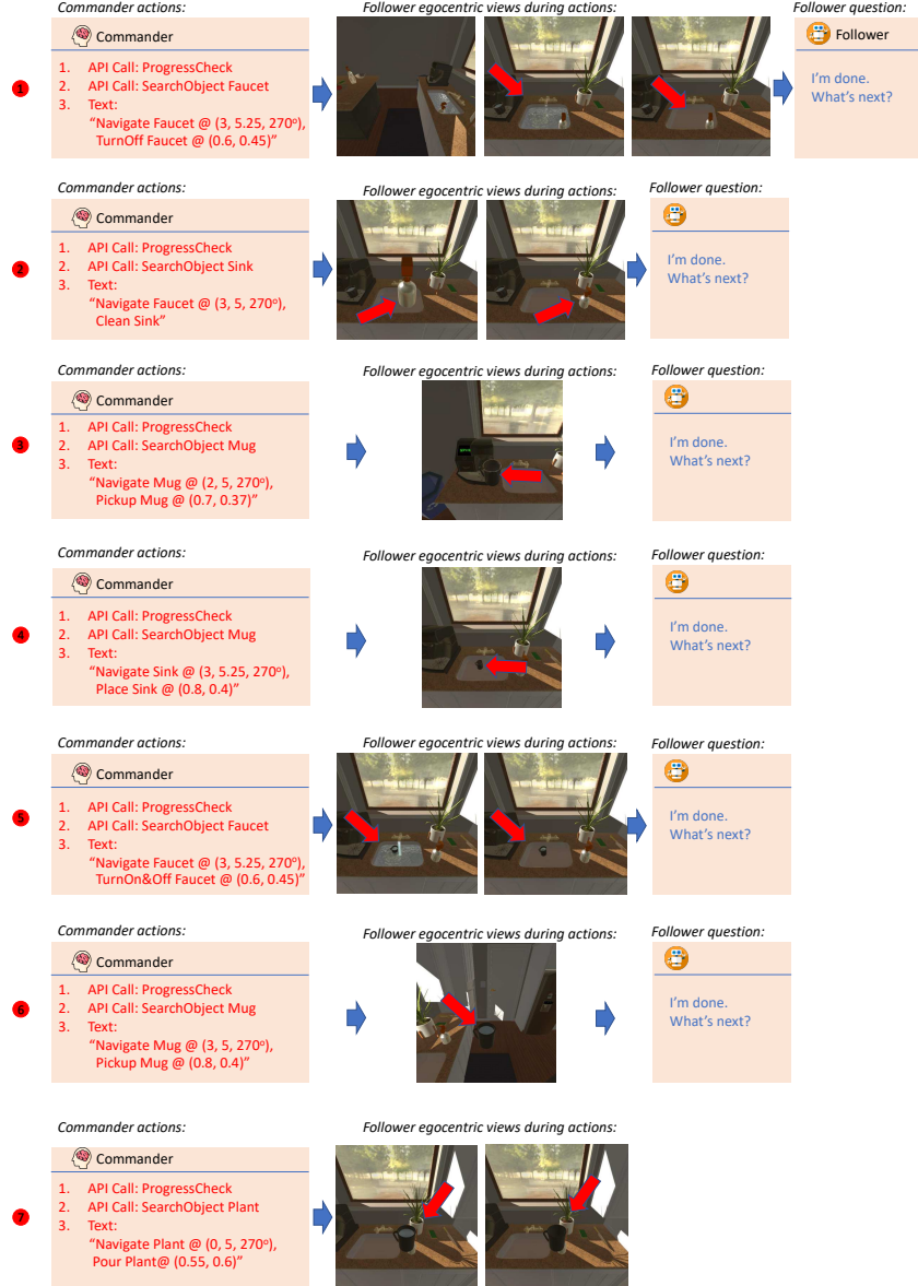
Figure B.3.: TATC "Water the plant" sequence. At each step the commander calls SearchObject to get an optimal navigation pose (e.g. ①: Navigate to Faucet @ (3, 5.25, 270°)), then uses ground-truth segmentation to compute an interaction target (e.g. ③: Pickup Mug @ (0.7, 0.37)). Steps 1–6 repeat for Faucet, Sink, Mug, Sink, Faucet, and Mug; step 7 pours water on the Plant @ (0.55, 0.6). After each sub-goal the follower executes in its egocentric view and reports completion.
