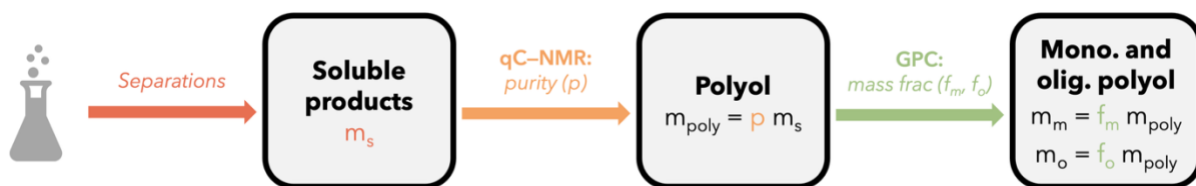
Figure 6.1. Separation and analysis methodology to quantify polyol monomer and oligomer mass of PUF glycolysis products.
