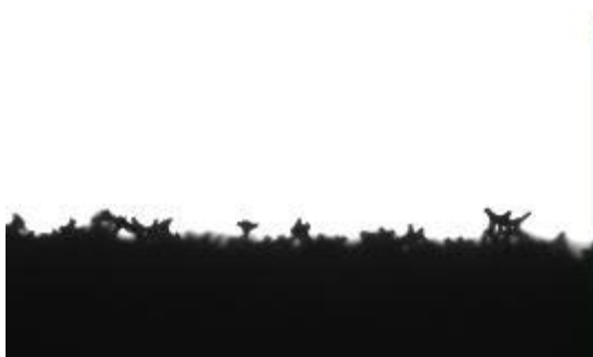
Figure 7.4. Photo of PUF surface, taken on ramé-hart model 100-00 goniometer, showing heterogeneity of surface used in contact angle measurements.
