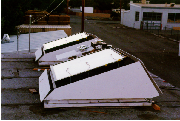
Figure 3. Test Sample Arrangements. (a) Setup for December Selective Double/Clear Double Tests. This photo was taken during tests of identical clear double skylights, but the differences in insulated glazing units would not be visible. In the December tests the Selective Double insulated glazing unit was installed in the far sample. (b) February Clear Double / Double Bubble Tests.
