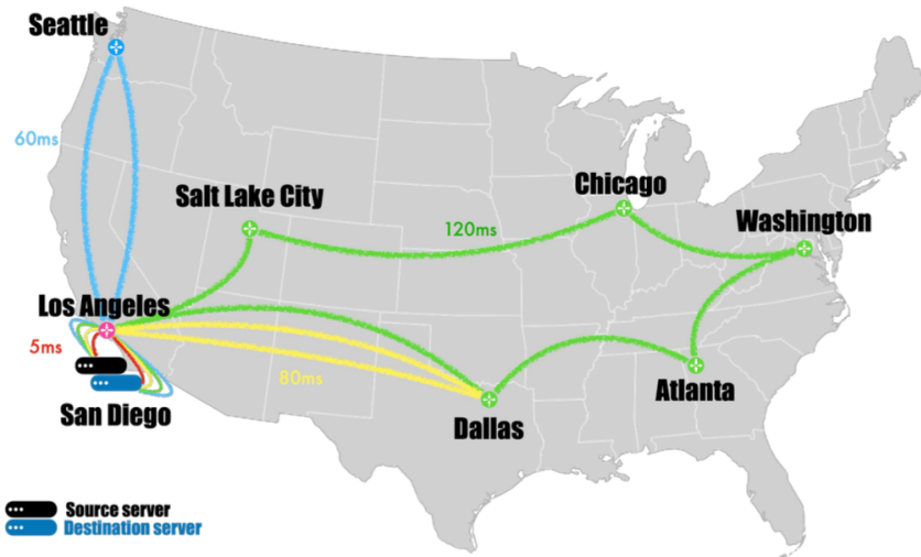
Figure 6.4. The variable-latency testbed: two co-located SDSC nodes interconnected through static routes across FABRIC, realizing round-trip times of 5-120 ms.
