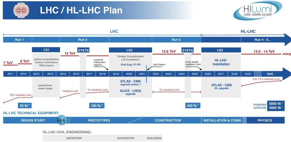
Figure 2.4. Timeline of the LHC runs and long shutdowns, with the energy and integrated luminosity of each, including the HL-LHC [27].
