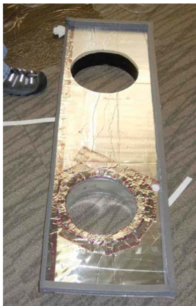
Figure 10: Duct Blaster manifold
