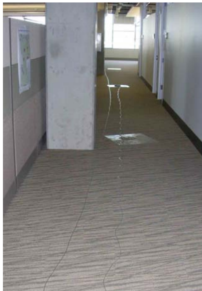
Figure 6: Installation of tubing for plenum pressure measurement
