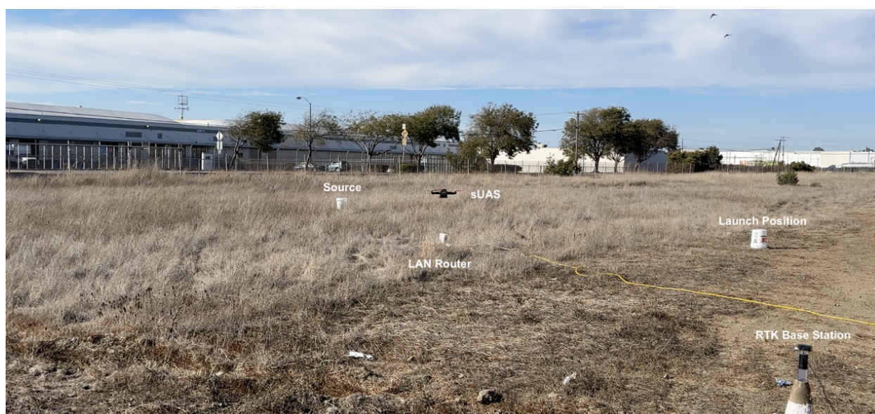
Figure 3.7: Setup for the 1 mCi ^{239}\text{Pu} -surrogate point source measurement. The source was placed on a 5-gallon bucket in an open field. A plastic scintillator integrated drone was flown to measure both the neutrons and gamma rays from the source.
