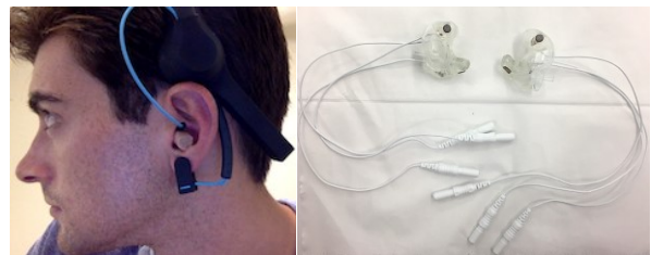
Figure 1. Recent BCI research in HCI has experimented with collecting and using electroencephalography (EEG) signals through noninvasive means, for example an earpiece that senses and uses brainwaves as an authentication method [15].
