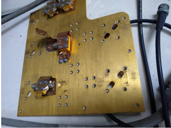
Figure C.1: Left: Their 12K plate. The components here are mechanically and thermally anchored with copper foil, held in place with washers and screws with a layer of indium foil for improved thermal contact. You can see the threads in the plate are stainless steel, press-in washers. Right: Another picture of their 12K plate, with the cryogenic amplifier included in the top right. It is anchored with a gold-plated copper block and screws.
