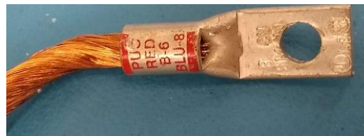
Figure C.2: Left: Picture of the packaging of the copper foil they use. Top: A homemade thermal strap soldered at one end and crimped to a ring terminal at the other. The twisted copper threads are from old speaker wire. Bottom: Close up of the crimping ring terminal they use.
