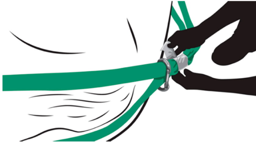
Figure A18. Place a carabiner between the loops going over the rump, and a piece of duct tape to secure temporarily the loops in place.
