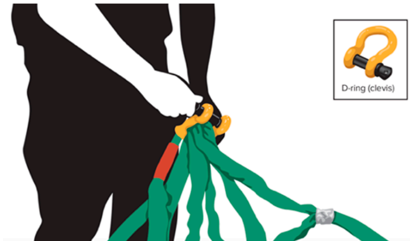
Figure A21. Place all four loops onto the clevis.
