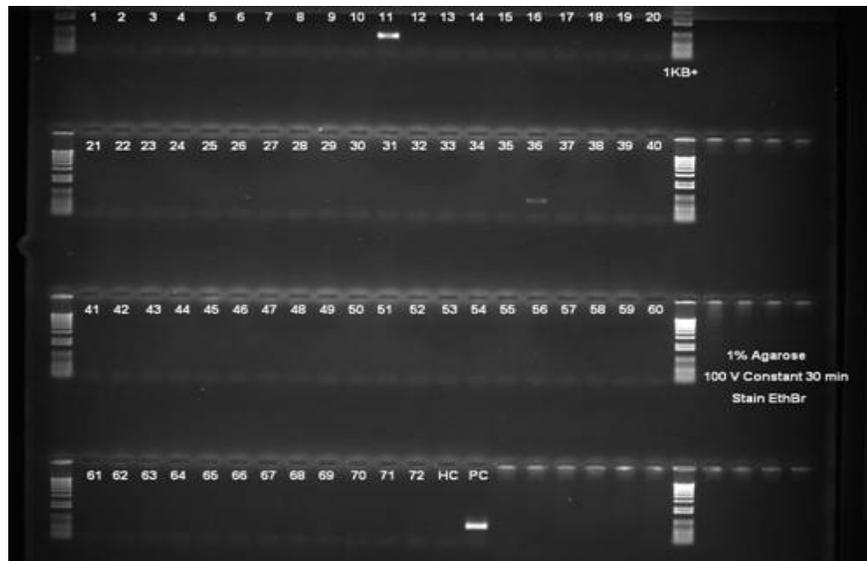
**Fig. 1.** Ethidium bromide stained agarose gel resulting from immunocapture reverse transcription polymerase chain reaction (IC-RT-PCR) of 72 samples, showing positive *Citrus tristeza virus* amplicons in samples 11 and 36. No other samples were found to be positive. HC = healthy control; PC = positive control. Primers targeting the CTV coat protein gene were used for the RT-PCR.
