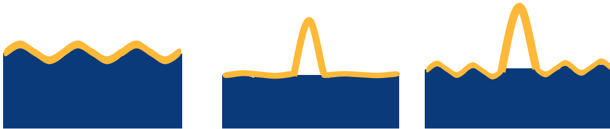
Figure 4.1: Deformation mechanisms in compressed thin films. From left to right: wrinkling with no delamination, buckling-driven interface delamination, concomitant wrinkling and buckle delamination
