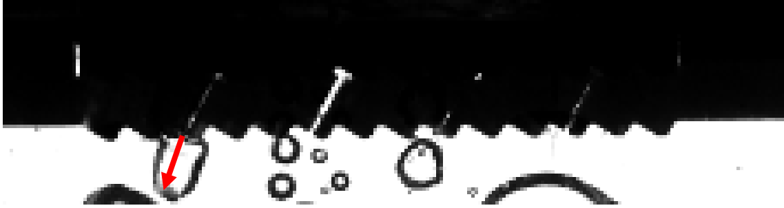
Figure 3-9: Height of the bubble in reference to the nucleation site angle
