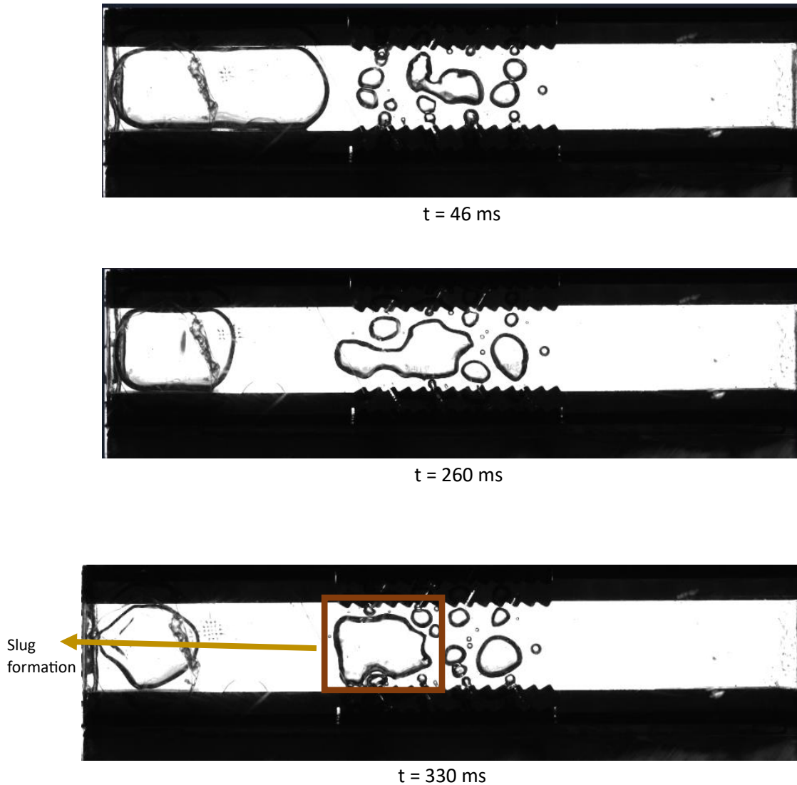
Figure 4-3: Sequence of frames at mid subcooling mid heat flux
