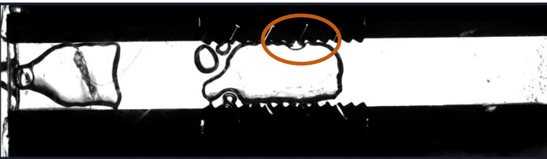
Figure 4-4: Sequence of frames at mid subcooling mid heat flux
