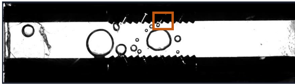
Figure 4-2: Sequence of frames at high subcooling mid heat flux
