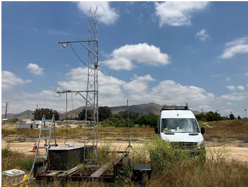
Figure 5.4. Experimental set up of side-by-side comparisons between 3-D sonic anemometer and mobile platform meteorological monitors
