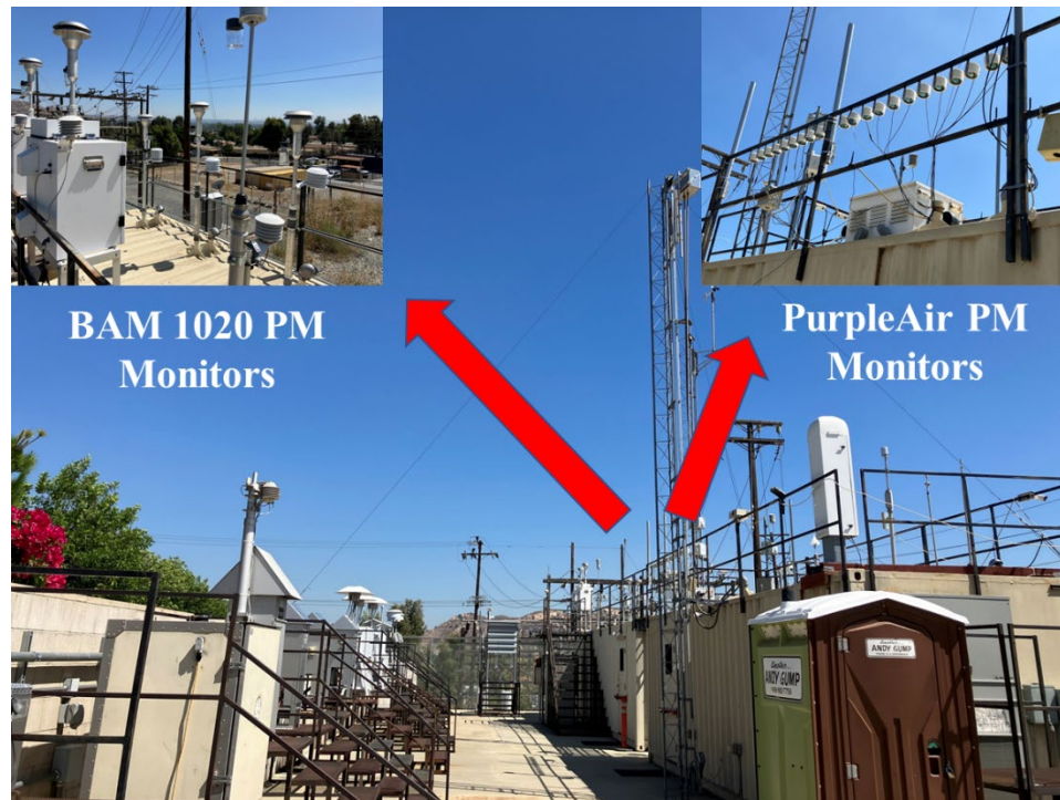
Figure 5.3. South Coast AQMD PM monitors setup at Rubidoux site
