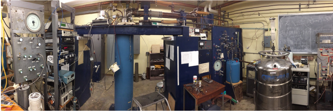
Figure 2.10: Panoramic picture of the low-temperature assembly. From left-to-right: Cell gas-handling system; Multi-level, portable shelving with temperature controllers and monitors, signal filter, pressure gauge, function generator, and oscilloscope; Vibration-isolation system with dewar; Pumping and filling lines for fridge, vacuum can, 1K pot, and dewar; Leak-detector and diffusion-pump assembly (behind the silver liquid-helium storage dewar); Portable ^3\text{He} - ^4\text{He} storage assembly with sealed pump.
