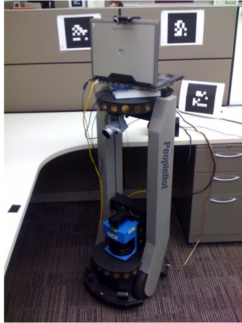
Figure 2.3: The robot platform used for these experiments. The webcam attached to the laptop is the one that is used to collect visual measurements.
