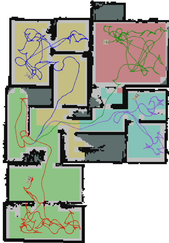
Figure 5.14: Sampling trajectory with four robots in one of our test environments. Partitions assigned to each robot are shown via shading open occupancy grid cells.
