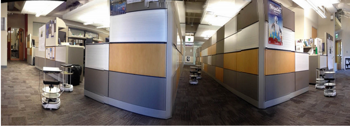
Figure 4.21: An example scenario for the experiments described in this paper. Three teams of two robots are exploring the branching hallway structure in an office environment. In this illustration, the robots are using the Divide and Conquer cooperative mapping strategy.
