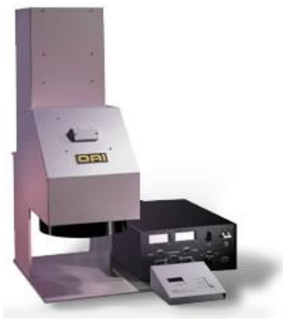
Figure 7. Light source for photolithography: OAI Model 30 UV light
