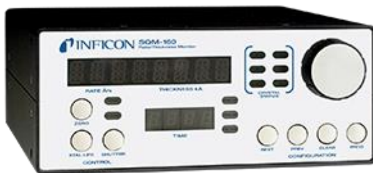
Figure 6. SQM-160 Thin Film Deposition Monitor
