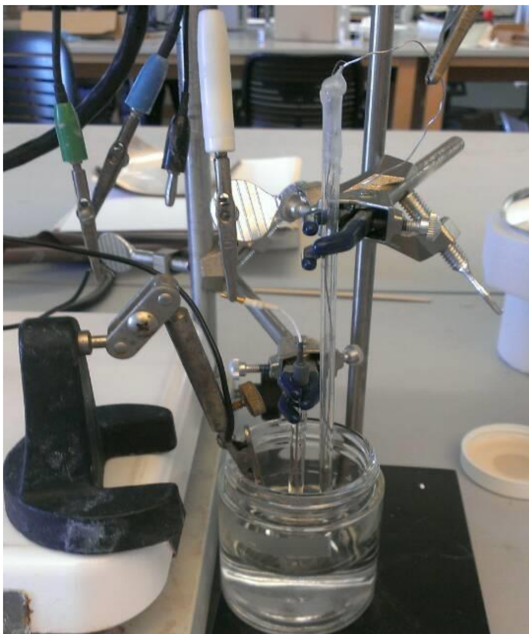
Figure 8. The set-up of the three electrode electrochemical cell
