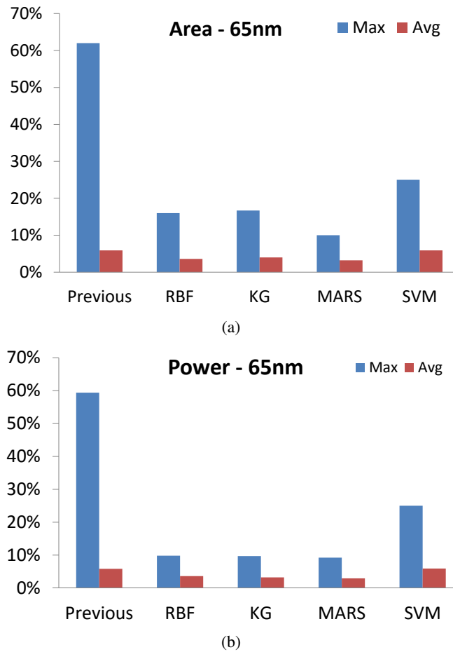
Figure 3.16: Comparison with estimation errors of “Previous” [116] in 65nm: (a) area and (b) power.
