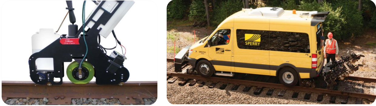
Figure 3.10: In-motion ultrasonic rail inspections using Rolling Search Units (RSUs).
