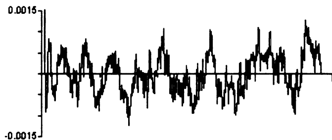
Figure 8. Stopped flow analysis of camphor. The absorbance change at 390 nm for camphor is able to be fit to a single exponential.
