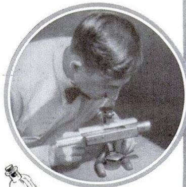
In circle, camera that makes records of film showing the inclination of well being dug. Right, whipstock that is set at bottom of well to deflect bit. Left, acid-etched bottle that shows slant of the well
