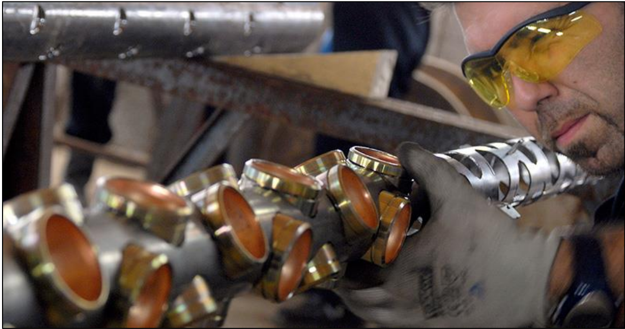
Figure 13: A Modern Perforating Gun.
