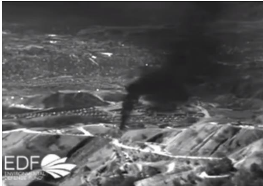
Figure 143: Infra-Red Image of Aliso Canyon Storage Facility Methane Leak, December 2015.
