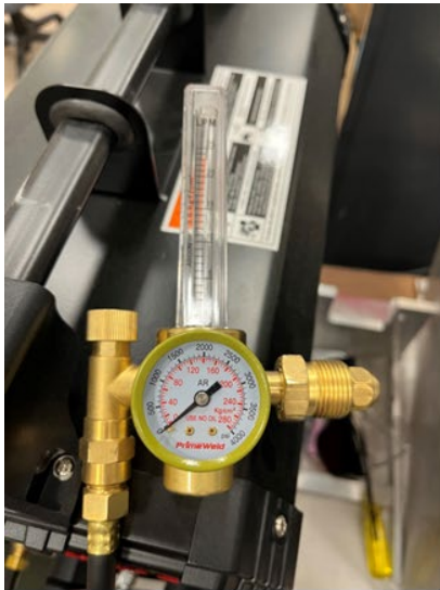
Regulator with flow meter
