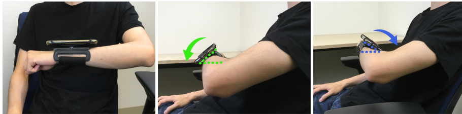
Figure 2.4: Tilt-based number picker: the user tilts the device away from the body (up) or towards the body (down) to increment and decrement a numeric value, respectively.
