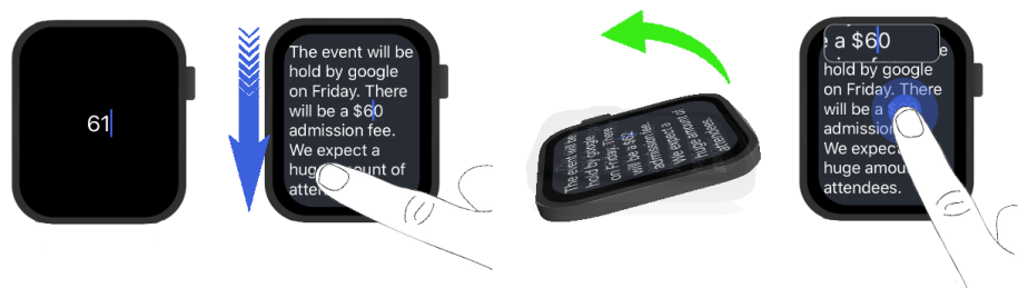
Figure 2.1: The four number pickers investigated in this work, from left: input stepper (the default number picker on most smartwatches), swipe (in this figure, the user is swiping down to decrease a value), tilt (in this figure, the user is tilting up to increase a value), and force (in this figure, the user is varying contact force to change a value). Unlike the default input stepper, the new methods do not display numeric values in full-screen when selected, instead display a magnifier window to display the value changing (see the last image).
