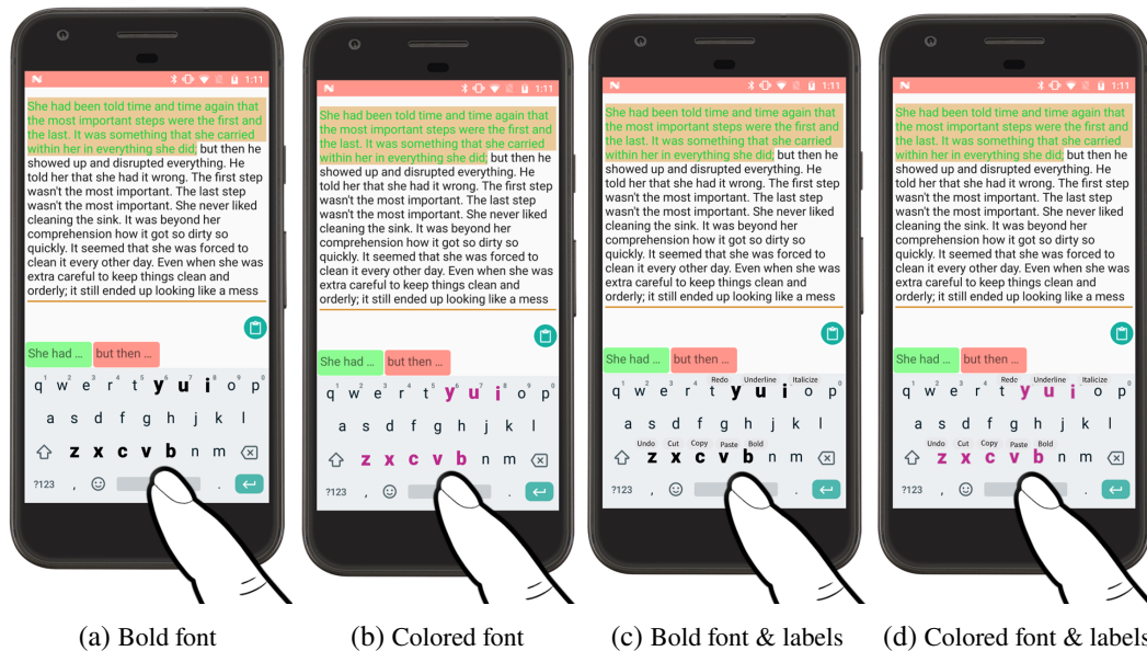
Figure 4.14: Four key highlighting approaches will be explored in the future to facilitate gestural shortcut discovery and learning.
