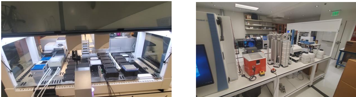
Figure 15. The Living Biofoundry. Tecan Liquid Handling systems (left) and ThermoFisher Laboratory Automation System (right). ThermoFisher TSQ Altis triple quadrupole liquid chromatography-mass spectrometer, bioreactors, and Illumina sequencers not shown.
