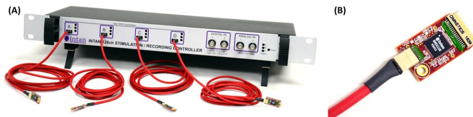
Figure 2.2: (A) Intan neuromodulation controller having four headstages (B) Intan headstage having two RHS2116 chip providing 32 channels in total.
