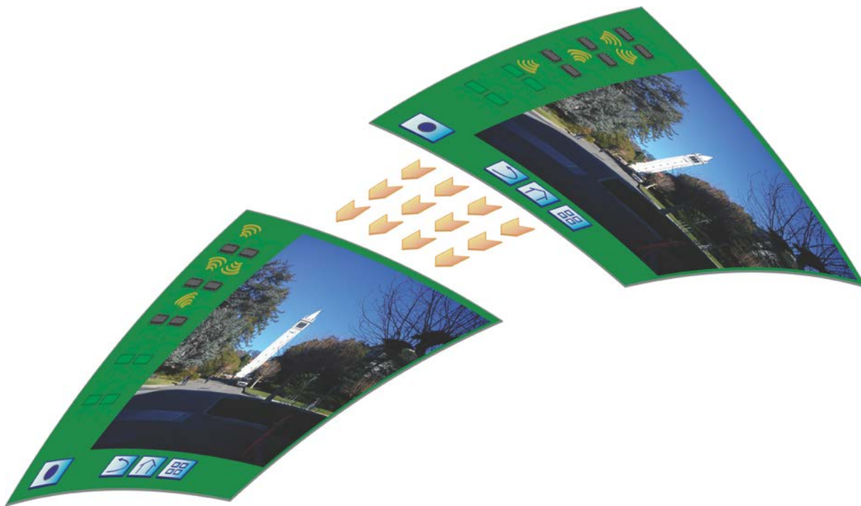
Figure 1.4. Flexible device can be upgraded by attaching two such devices and the chips communicate with each other wirelessly
