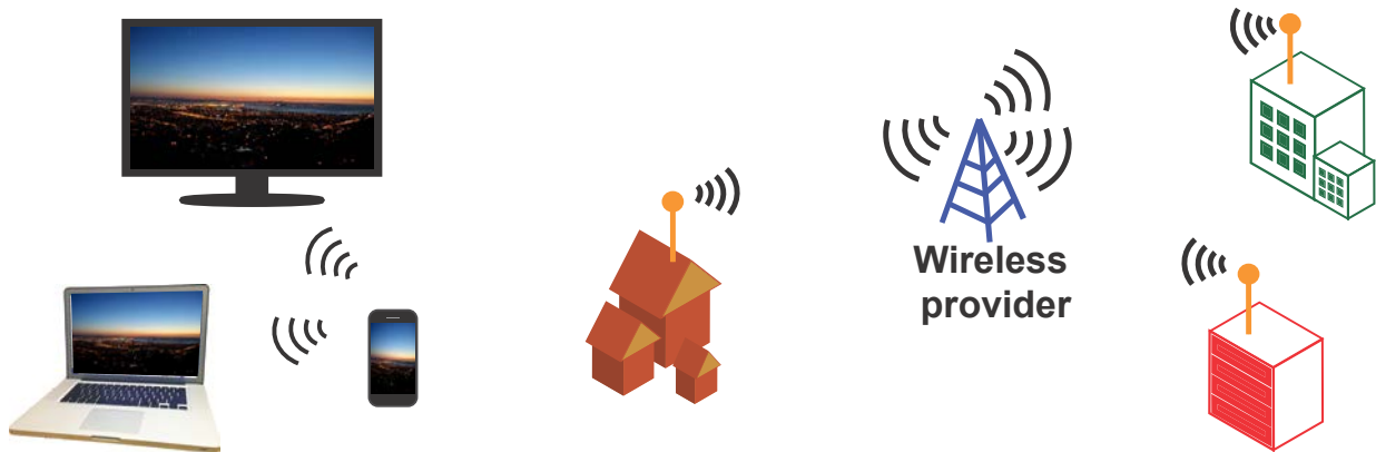
Figure 1.2. Millimeter-wave/terahertz networks for personal area networks [left] and wireless backhauls [right]
