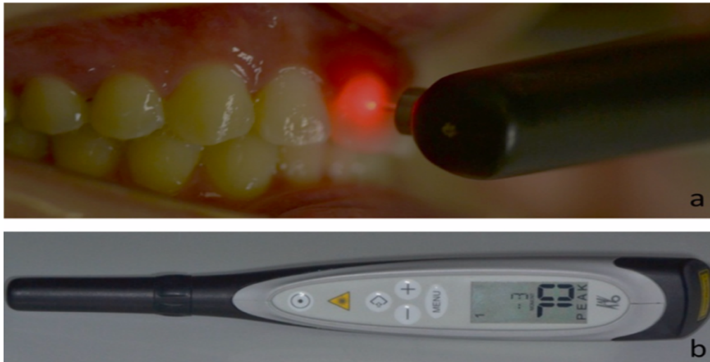
Figure 4- DIAGNOdent pen. (a) Use for WSL detection. (b) device calibrated to use[28]
