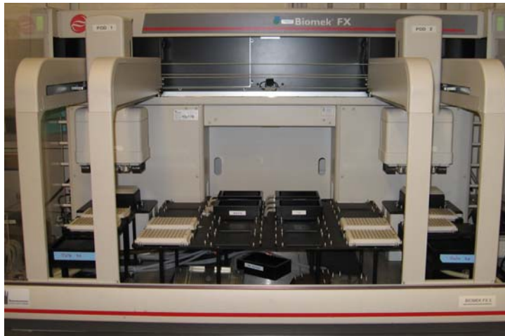
Figure 3: Biomek FX automated pipetting instrument. Dual Multi-channel pipette heads.
