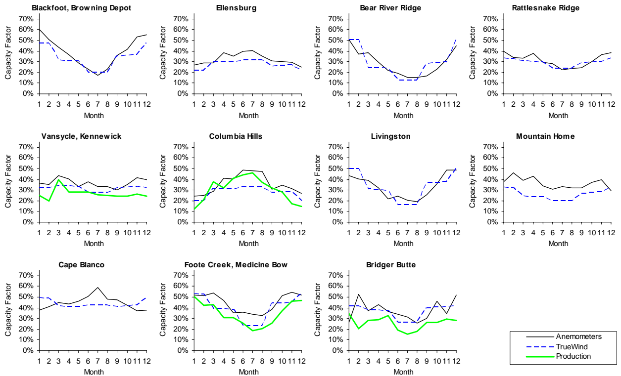
Figure 37. Monthly Average Capacity Factor For Each Resource Area from Anemometers and TrueWind Data at the Same Grid Cell, and Production Turbines in the Same Region (Northwest)
