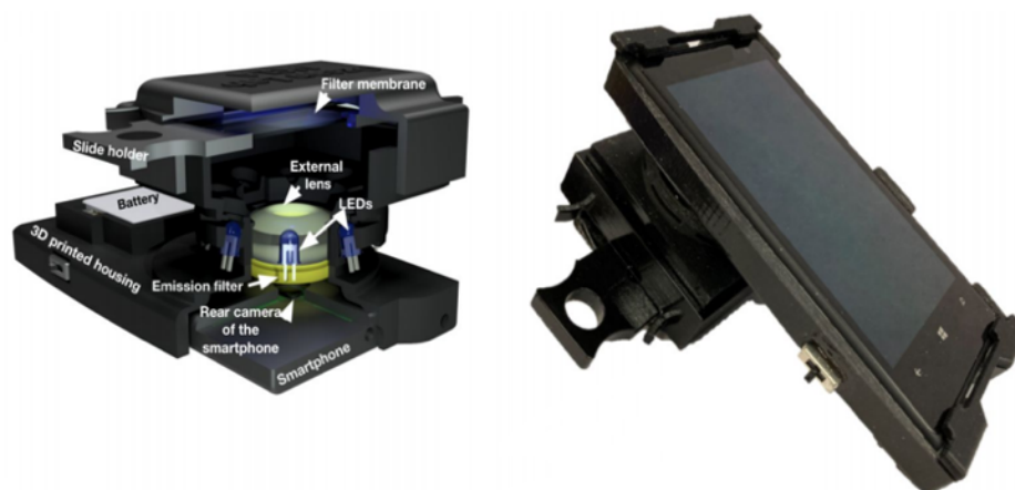
Figure 5-2. The prototype used for imaging of the membranes with microplastics samples
