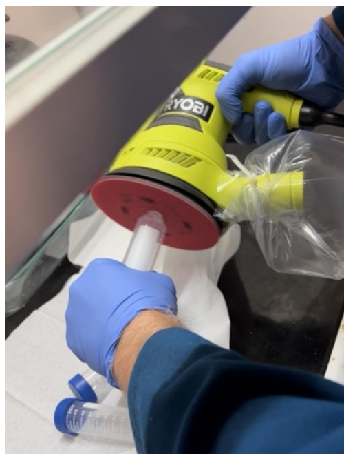
Figure 7-1. Creation of microplastics using an orbital sander with an attachment to catch created particles.
