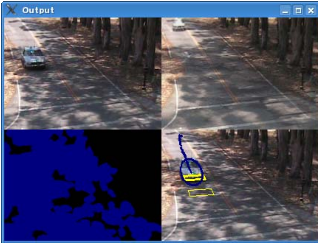
Figure 3.11. Vehicle tracking with virtual loop matched with real loop on the ground
