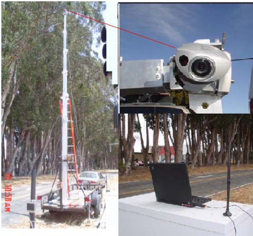
Figure 3.2. Video Camera Mounting on Mobile Trailer: Left: Mobile retractable pole; Upper right: PTZ camera on top for looking at the loop and for vehicle tracking to obtain baseline data; Lower right: video computer also running IEEE 802.11b wireless communication using USB port.
