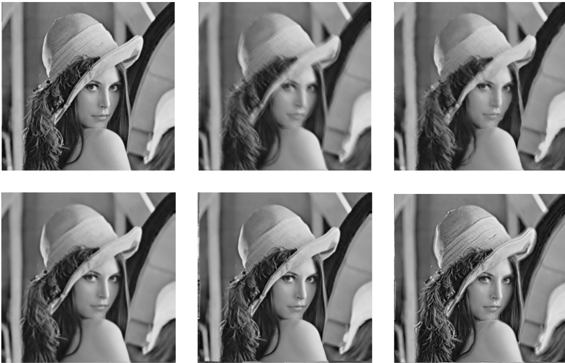
Figure 4.2: Geometric distortion correction. Top, left to right: true image, mean of 10 input frames, median of 10 input frames. Bottom, left to right: Variation 1 reconstruction, Variation 2 reconstruction, geometric distortion correction using [MG12].
