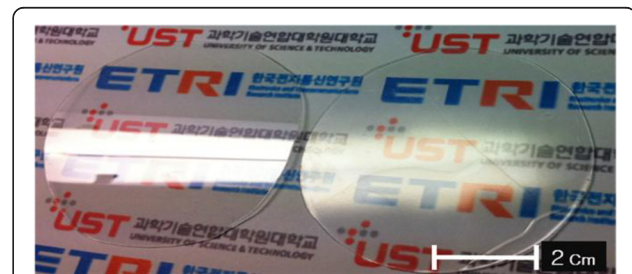
Figure 6 Digital images of the bare PC film (left) and the AR nanostructured PC film (right).
