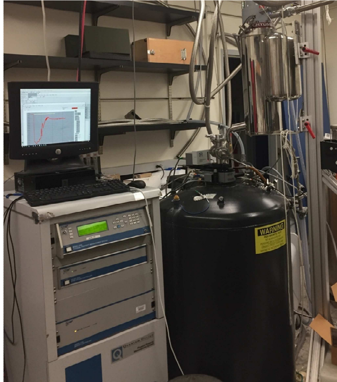
Figure 2.1. Quantum Design PPMS fitted with a Cryomech HeRL15 helium reliquefier.
