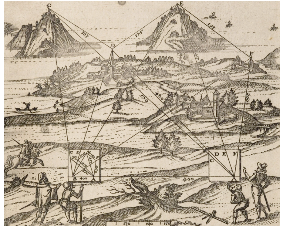
Renaissance chorographic survey of a region. Leonhard Zubler, 1607. De Instrumenti usu in describendis quatuor Pagis: & quantum hi à se distent. Fabrica et vsus instrvmenti chorographici: qvo mira facilitate describuntur regiones & singulae partes earum, veluti Montes, Vrbes, Castella, Pagi, Propugnacula, & simila (Creative Commons License 2016, Max Planck Institute for the History of Science, Library).
