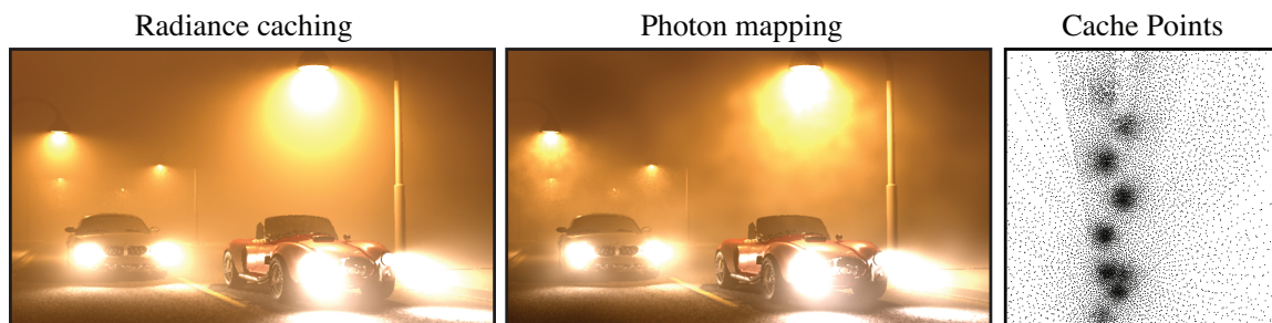
Figure 5.16: A equal-time, contrast-enhanced comparison between radiance caching and photon mapping in the cars scene from Figure 5.15. The scene has a large extent, making it difficult to render with methods such as photon mapping that compute scattering in the entire medium. Artifacts remain in the homogeneous medium even after storing 8M photons. On the right we show a horizontal cross section of the single scattering cache points as seen from above. In this visualization, the camera is located at the bottom looking up. Note the concentration of cache points around the street lights and headlights near the camera. The error tolerances were set at 0.25 and 0.75 for the single and multiple scattering caches, respectively.
