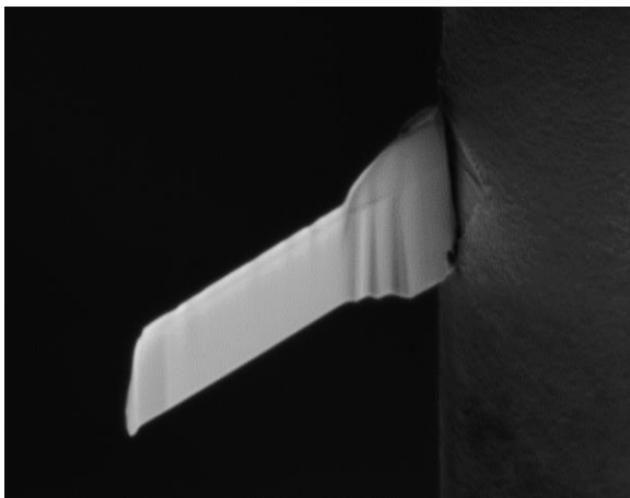
Figure 2.26 – An electron-transparent sample ready for STEM
